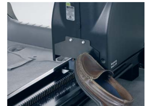
Safety plate obstruction sensor.
