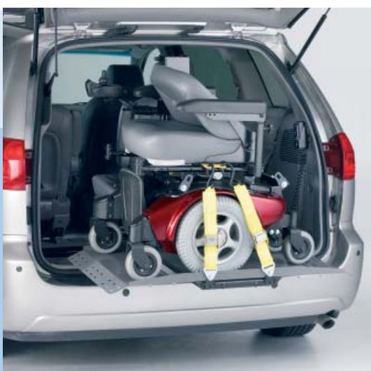
Once the wheelchair is secured to the platform you just press the hand control button and the lift does all the work.
