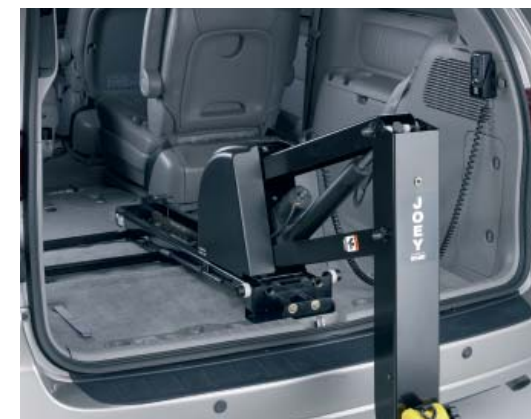
The compact rail design uses only the third row seat fixings in the floor.
